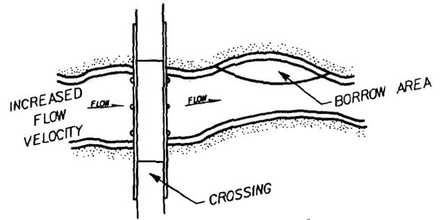
Figure 5-41. Material removal.
