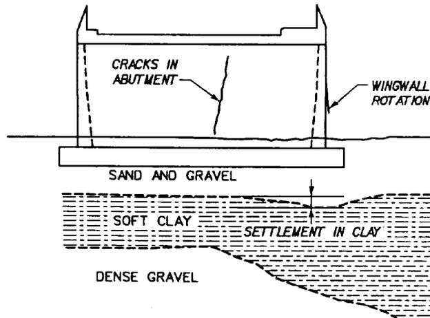
Figure 5-19. Differential settlement under an abutment.
