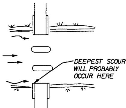
Figure 5-35. Protruding abutments.
